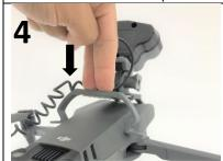
Push down the back side of the Head-Unit bracket, it will flex and slide to lock over the drone's body
