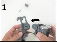
Remove the bolt and nut from the Head-Unit Bracket and slide the LEDs Head-Unit into place
