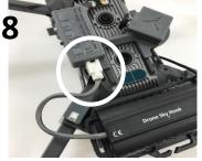
Connect the GREY wire plug to the Sky Hook PLUS - AUX CON port and verify it is locked in place
