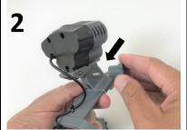
Install the bolt and nut in the Head-Unit, set to desired angle and tighten the nut (only by hand)
