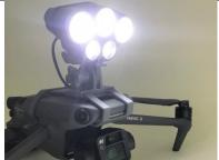
Operation when combined with the Sky Hook Release PLUS device: Turn ON the Sky Hook's AUX Port to set the Searchlight ON.
