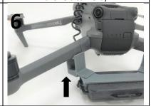
Align the Battery Pack mounting section below the drone's back arms and slide **UP** until it locks
