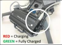
**CHARGING:** Connect the Micro USB cable to the battery-pack and to a USB charger
