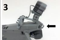
Slide back the Head-Unit from the drone's front-end (above the drone's camera)
