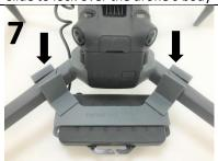
Verify that both sides of the Battery Pack are locked over the drone's rear arms and that the Battery Pack in centered
