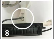
Connect the GREY wire plug to the Sky Hook's AUX CON port and verify it is locked in place
