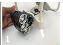
Slide the **FRONT SIDE** of the LED bracket over the **FRONT RIGHT** landing gear until it locks in place
