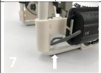
Route the **GREY** wire between the Battery-pack bracket and the landing gear
