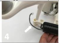
Slide the **FRONT SIDE** of the Battery-pack bracket over the **FRONT LEFT** landing gear until it locks in place
