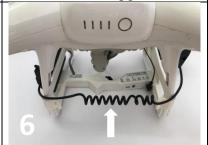
Verify that the spiral wire is routed **BEHIND both REAR landing gears**
