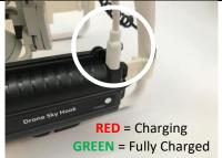
**CHARGING:** Connect the Micro USB cable to the battery-pack and to a USB charger
