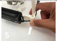
Slide the **REAR SIDE** of the Batterypack bracket over the **REAR LEFT** landing gear until it locks in place
